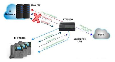
When FTA5120 receives calls, it will search the internal SAS registration database to locate the destination address (according to AOR or Contact). If the destination address is not found, FTA5120 will forwards the call to itself. FTA5120 has two FXO port, enterprise can preserves its capability for outgoing calls (from UAs to the PSTN network) or convey IP calls through PSTN line (Via SIP Trunk).
