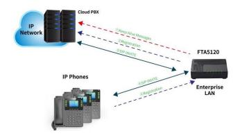
In Normal state, FTA5120 receives REGISTER request and SIP Invite from UAs in the network and will forward them to the external proxy (i.e., outbound server, proxy server), and send SIP Option message to the cloud PBX to detect its status. Once the proxy replies with a SIP 200 OK, the device records the Contact and Address of Record (AOR) of the UAs in its internal SAS registration database. FTA5120 will maintain a database of all the registered UAs in the network.
